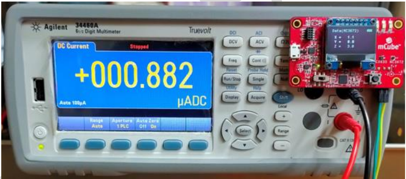
Figure 22 Wake supply current @ ultra-low power, 25Hz
