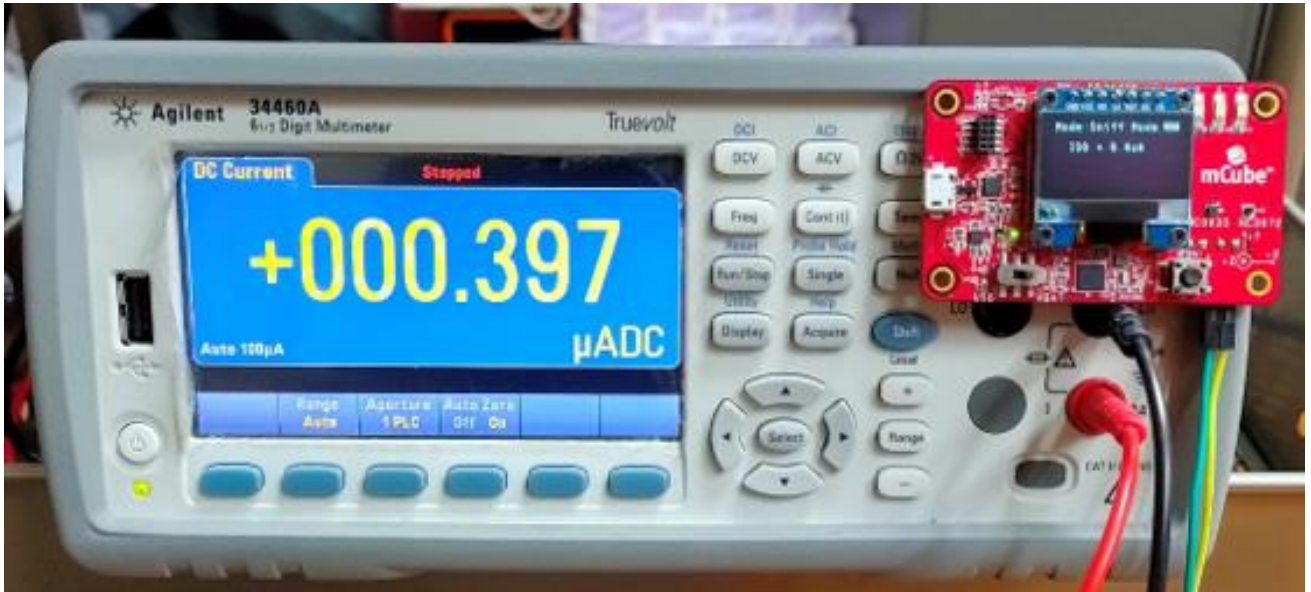
Figure 21 Sniff current at 6Hz
