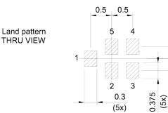
Landing pad tolerance -0.02 **Figure 2:** Drawing of package with package height A = 0.45 mm (max.). See Sec. Package information (p. 18).
