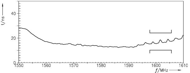
Figure 7: Group delay ripple.
