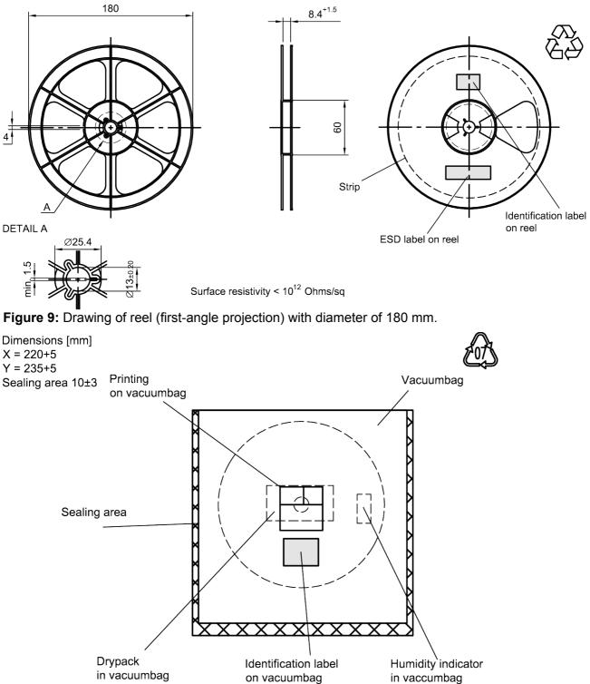
Figure 10: Drawing of moisture barrier bag (MBB) for reel with diameter of 180 mm.
