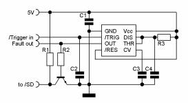
Figure 16: Fault Timer circuitry with LMC555
