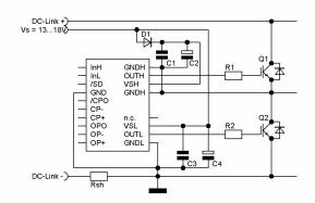
Figure 11: Ground reference at low side emitter
