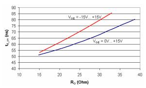
Figure 7: Comparison  $t_{d_on} = f(R_G)$
