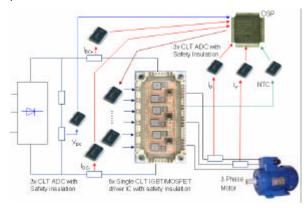
Figure 18: Application with ADC's and driver IC's of eupec EiceDRIVER<sup>™</sup> family
