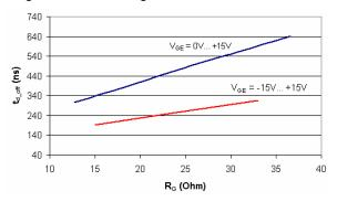
Figure 8: Comparison  $t_{d_{off}} = f(R_G)$
