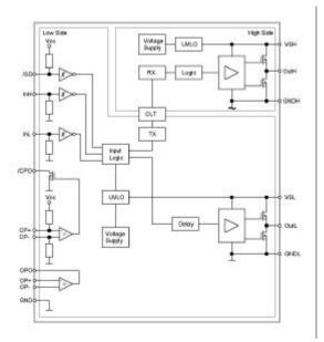
Figure 2: Block diagram of 2ED020I12-F
