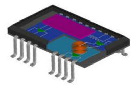
The 2ED020I12-F contains two drivers for an IGBT or MOSFET half-bridge, whereby the high side is galvanically isolated from the low side part through a coreless transformer system as described before. The main features of the IC are:
