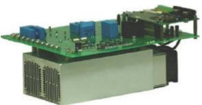
Figure 9: 15kVA converter with 2ED020I12-F
