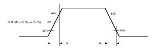
Figure 3. CML Output Transition Times
