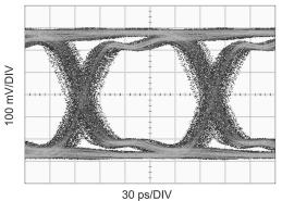
Figure 13. Equalized Signal (40 In FR4, 6.4 Gbps, PRBS7, 0x06 Setting)
