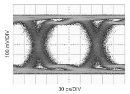
Figure 14. Equalized Signal (40 In FR4, 6.4 Gbps, PRBS31, 0x06 Setting)
