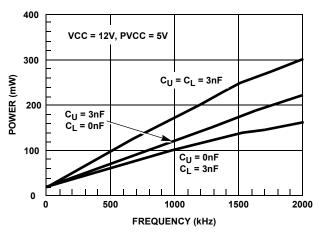
FIGURE 5. 3nF LOADING PROFILE (HIP6603B)
