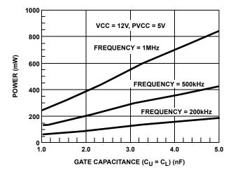
FIGURE 7. POWER DISSIPATION vs FREQUENCY (HIP6601B)
