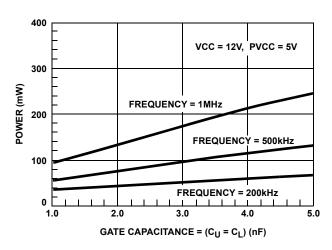
FIGURE 6. VARIABLE LOADING PROFILE (HIP6603B)
