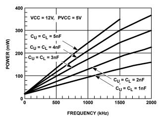
FIGURE 4. POWER DISSIPATION vs FREQUENCY (HIP6603B)
