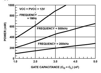
FIGURE 3. POWER DISSIPATION vs LOADING
