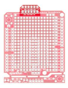
If you decide that you want to connect a different serial UART device or use different pins for serial, we added closed jumpers on the back. Simply cut the traces and reroute the connection by adding wires to the headers.
