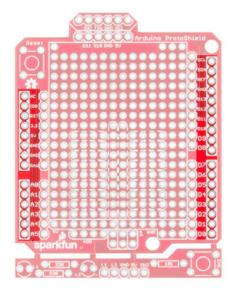
These pins are also broken out on the other side of its labeling. You will notice that the 1x10 header on the upper right side of the board is slightly offset from the Arduino R3 footprint. Don't worry, this was intentional so that you can place the board on a standard breadboard!
