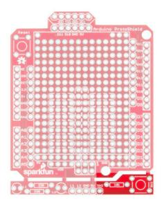
**Note:** The button **(SW2)** is not connected **(NC)**. To control, simply solder a wire from **SW2** to an I/O pin. 5V and ground are currently connected to the rest of the shield between the mousebites. We left it up to the user to connect.
