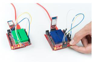
**Note:** Take turns pressing on the push buttons to transmit. The message may get garbled when both bluetooths are transmitting simultaneously.
