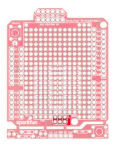
Note: The MISO, MOSI, and SCK pins are not connected (NC).
