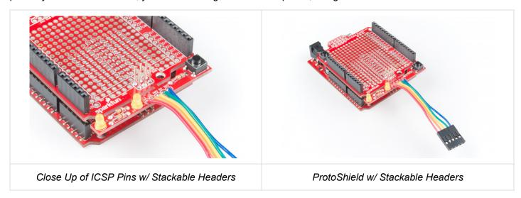
**♦ Oh snap!** This shield was designed for the Arduino Uno footprint. If you are using a variant with 3.3V logic level on the ICSP pin (i.e. SAMD21 Development Board or Arduino Pro 3.3V/8MHz), you will need to cut the two traces connecting to the 5V pin on the 1x3 ICSP header.
