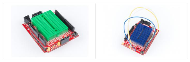
For those sandwiching the ProtoShield with another shield, you can solder two 1x3 stackable headers for the ICSP pins. If you choose this route, you will need to go with a lower profile, using wires to connect the circuit.
