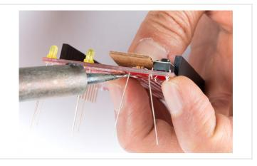
Check Alignment Before Soldering Away!
