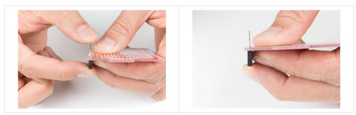
Grab the soldering iron with your soldering hand and tack on one pin. Repeat for each header.
