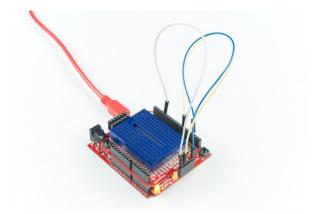
Let's connect L2 to pin 6 and to fade in and out. Assuming that you soldered to L2, connect it to pin 6.
