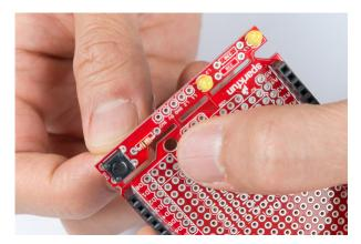
Bend the terminals to hold the resistor in place for soldering. The resistor can get hot to the touch when holding the component down during soldering. At this point, feel free to grab a small piece of cardboard to hold the resistor down. When you are ready, tack one of the  $10k\Omega$  resistor's pins. Repeat for the  $330\Omega$  resistors.
