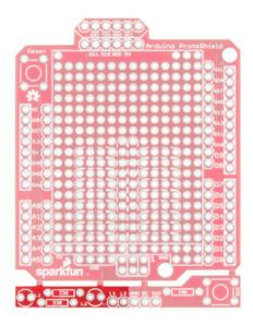
**Note:** The LED pins **L1 and L2 are not connected (NC)**. To control, simply solder a wire from **L1** or **L2** to an I/O pin. Ground is currently connected to the rest of the shield between the mousebites. We left it up to the user to choose and solder these connections.
