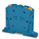
High-current terminal block, nom. voltage: 1000 V, nominal current: 232 A, connection method: Power-Turn connection, 1 level, cross section: 25 mm<sup>2</sup> - 95 mm<sup>2</sup>, mounting type: direct screw connection, color: blue
