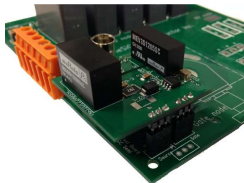
Figure 5: GeneSiC Gate Drive Board (GA03IDDJT30-FR4) connected to the Test Board's Gate Drive Connection
