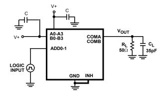
FIGURE 2A. t<sub>BBM</sub> MEASUREMENT POINTS
