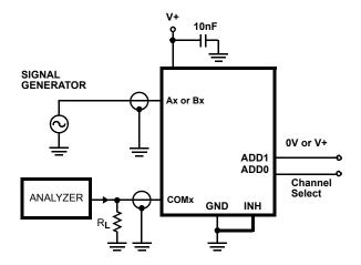
Off-Isolation is measured between COM and "Off" NO terminal on each switch.
