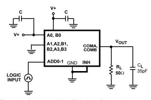
Repeat test for other switches. C<sub>L</sub> includes fixture and stray capacitance.
