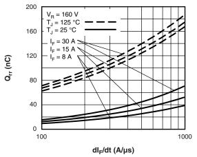
Fig. 8 - Typical Stored Charge vs. dI<sub>F</sub>/dt
