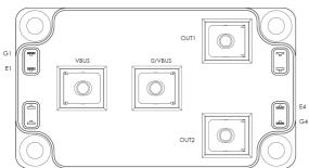
$V_{CES} = 600V$  $I_{C} = 180A$  @  $T_{C} = 80^{\circ}C$
