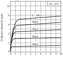
Collector-emitter voltage  $V_{CE}$  (V)
