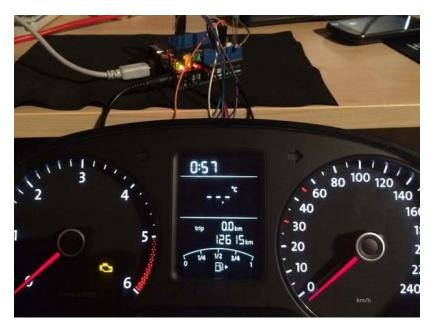
Ever wanted to play a car/truck simulator with a real dashboard on your PC? Me too! I'm trying to control a VW Polo 6R dashboard via CAN Bus with an Arduino Uno and a Seeed CAN Bus Shield. Inspired by Silas Parker. Thanks Sepp and Is0-Mick for their great support!
