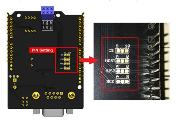
• Step2: Cut the wire between pad9 and the middle pad.
