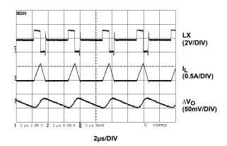
FIGURE 12. PFM STEADY-STATE OPERATION WAVEFORM (I<sub>O</sub> = 100mA)
