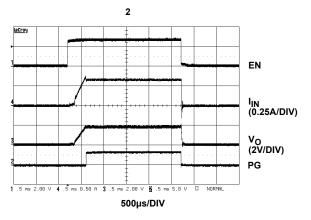
FIGURE 11. ENABLE AND SHUT-DOWN
