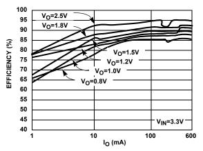
FIGURE 3. EFFICIENCY vs I<sub>O</sub> (PFM/FWM MODE)
