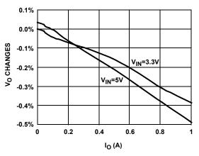
FIGURE 6. LOAD REGULATIONS (PWM MODE)
