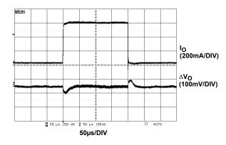
FIGURE 17. PWM LOAD TRANSIENT RESPONSE (30mA TO 600mA)
