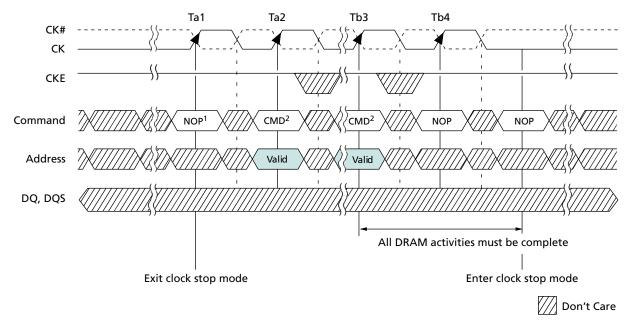
Notes: 1. Prior to Ta1, the device is in clock stop mode. To exit, at least one NOP is required before issuing any valid command.
