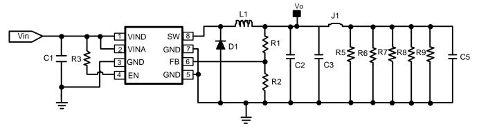
Figure 1. LM2832Y 8-Pin MSOP-PowerPAD Demo Board Schematic
