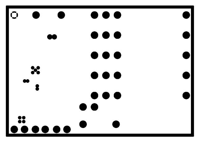
Figure 4. Internal Plane 2 (V<sub>IN</sub>)
