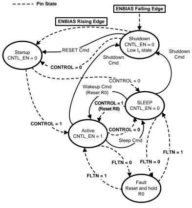
Figure 17. LM10520 State Diagram
