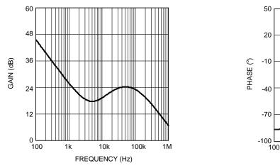
Figure 29. Error Amp. Gain and Phase
