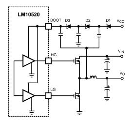
Figure 25. Charge Pump with Added Gate Drive
