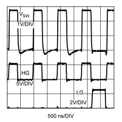
Figure 19. Output Pre-Bias Mode Waveforms
