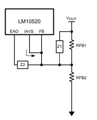
Figure 15. Connecting IAVS to the Feedback Node
