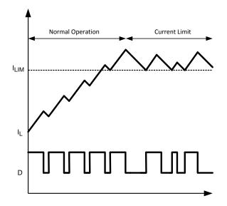
Figure 26. Current Limit Threshold
