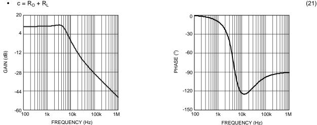
Figure 28. Power Stage Gain and Phase
