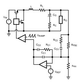
Figure 27. Power Stage and Error Amp
