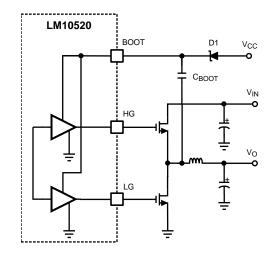
Figure 23. Basic Charge Pump (Bootstrap)
