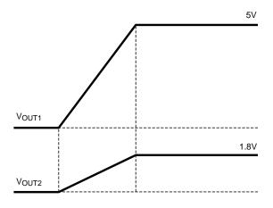
Figure 21. Tracking with Equal Soft-Start Time
