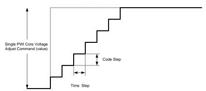
Figure 16. Digital Slew Rate Control
