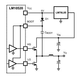
Figure 24. LM78L05 Feeding Basic Charge Pump
