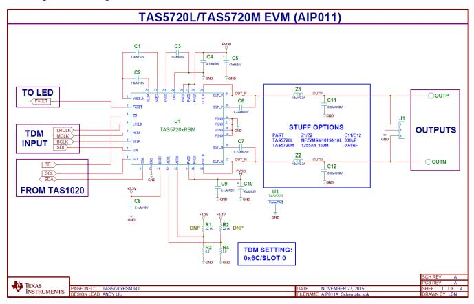
Figure 6-1. TAS5720MEVM Schematic (1 of 2)
