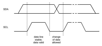
Figure 16. Bit Transfer on the I<sup>2</sup>C-Bus
