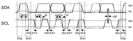
Figure 4. I<sup>2</sup>C Interface Timing Diagram
