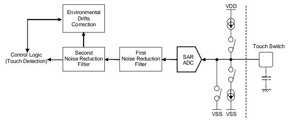
Figure 5. Touch Sensor Block Diagram
