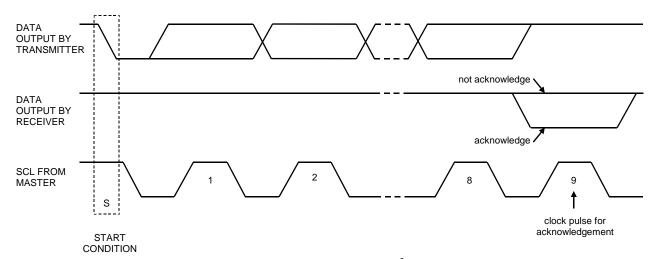
Figure 15. Acknowledge on the I<sup>2</sup>C-Bus
