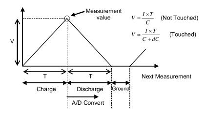
Figure 6. The Voltage Transaction of a Sense Terminal
