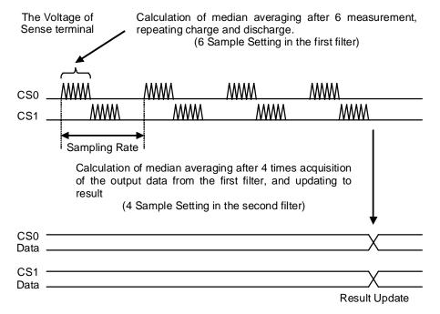
Figure 7. The Measurement of a Sense Terminal and The Data Update
