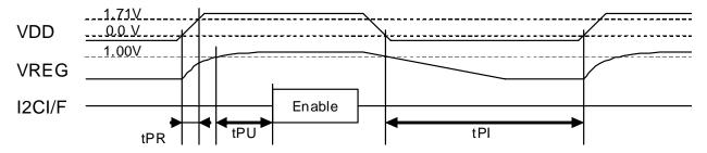
Figure 3. Power up Timing Diagram
