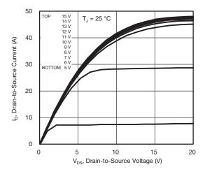
Fig. 1 - Typical Output Characteristics
