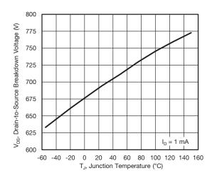
Fig. 11 - Temperature vs. Drain-to-Source Voltage
