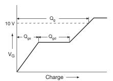
Fig. 17 - Basic Gate Charge Waveform
