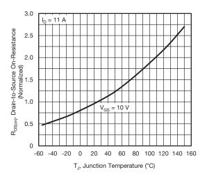
Fig. 4 - Normalized On-Resistance vs. Temperature
