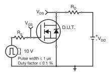
Fig. 13 - Switching Time Test Circuit
