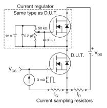
Fig. 18 - Gate Charge Test Circuit
