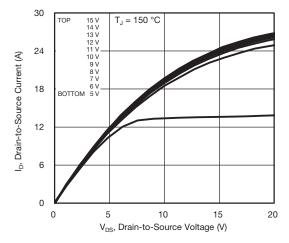
Fig. 2 - Typical Output Characteristics
