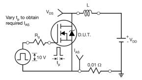
Fig. 15 - Unclamped Inductive Test Circuit
