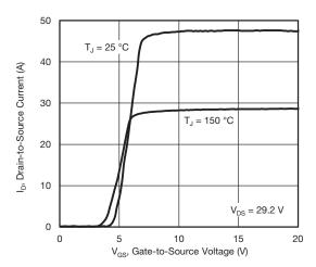
Fig. 3 - Typical Transfer Characteristics
