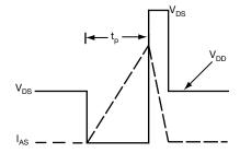
Fig. 16 - Unclamped Inductive Waveforms
