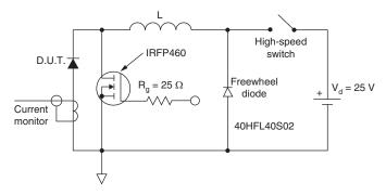
Fig. 8 - Unclamped Inductive Test Circuit
