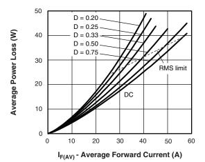
Fig. 6 - Forward Power Loss Characteristics (Per Leg)
