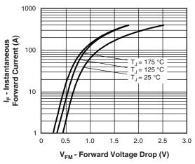
Fig. 1 - Maximum Forward Voltage Drop Characteristics (Per Leg)
