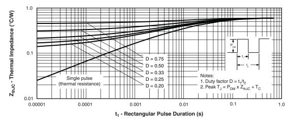
Fig. 4 - Maximum Thermal Impedance  $Z_{thJC}$  Characteristics (Per Leg)
