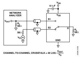
Figure 26. Channel-to-Channel Crosstalk
