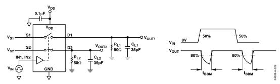
Figure 22. Break-Before-Make Time Delay, tbbm (ADG813)
