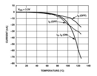
Figure 9. Leakage Currents vs. Temperature,  $V_{DD} = 3.3 \text{ V}$
