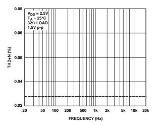
Figure 17. Total Harmonic Distortion
