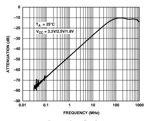
Figure 15. Crosstalk vs. Frequency
