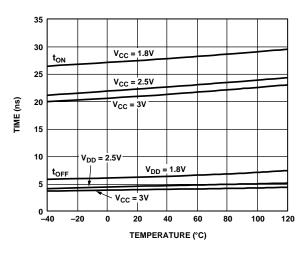
Figure 13. ton/toff Times vs. Temperature
