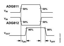
Figure 21. Switching Times
