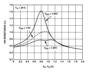
Figure 5. On Resistance vs.  $V_D$  ( $V_S$ ),  $V_{DD}$  = 1.8 V ± 0.15 V
