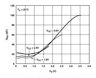
Figure 12. Charge Injection vs. Source Voltage
