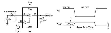
Figure 23. Charge Injection
