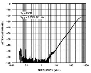
Figure 16. Off Isolation vs. Frequency
