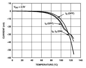
Figure 10. Leakage Currents vs. Temperature,  $V_{DD} = 2.5 V$
