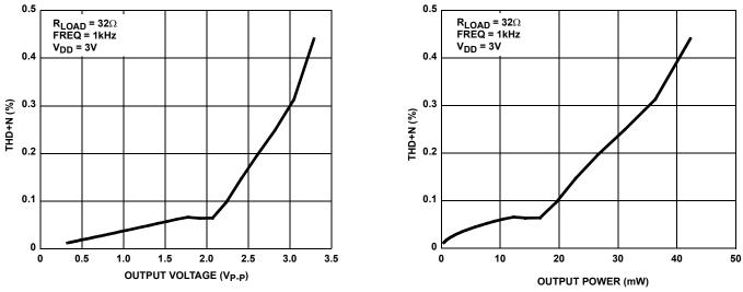
FIGURE 12. THD+N vs OUTPUT VOLTAGE
