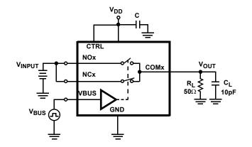
Repeat test for all switches.  $\mathbf{C}_{\mathsf{L}}$  includes fixture and stray capacitance.
