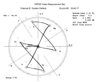
FIGURE 9. VECTOR-SCOPE PLOT AFTER SWITCH
