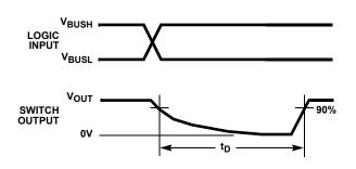
FIGURE 2A. MEASUREMENT POINTS
