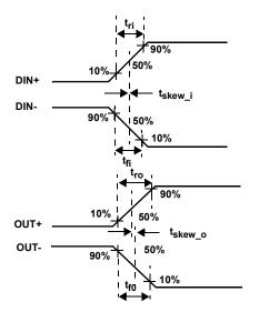
FIGURE 7A. MEASUREMENT POINTS
