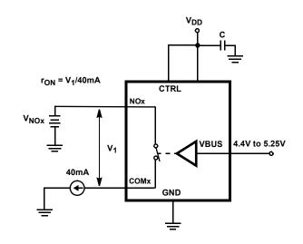
Repeat test for all switches. FIGURE 4. USB r<sub>ON</sub> TEST CIRCUIT
