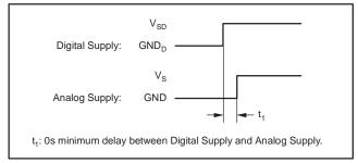
Figure 7. Power Supply Timing Requirements
