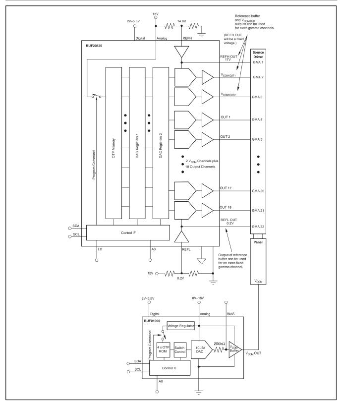
Figure 17. 22-Gamma Channel Solution
