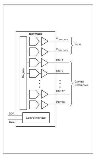
Figure 14. BUF20820 Used for Programmable V<sub>COM</sub>
