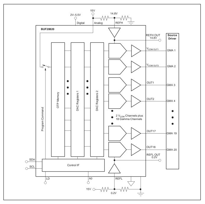
Figure 16. 20-Gamma Channel Solution—2 V<sub>COM</sub> Channels Used as Additional Gamma Channels
