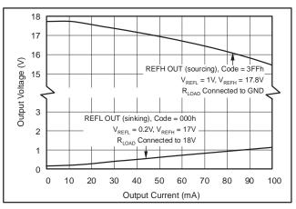
Figure 15. Reference Buffer Output Voltage vs Output Current
