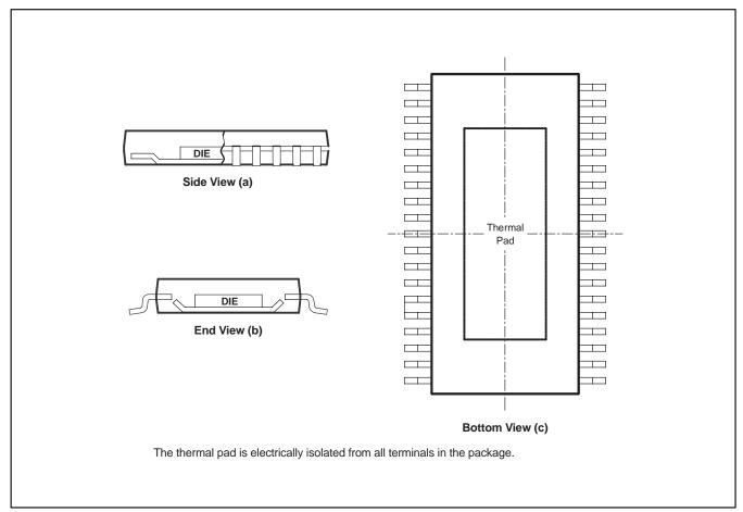
Figure 23. Views of Thermally-Enhanced DCP Package
