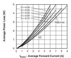
Fig. 6 - Forward Power Loss Characteristics
