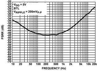
FIGURE 7. PSRR vs FREQUENCY
