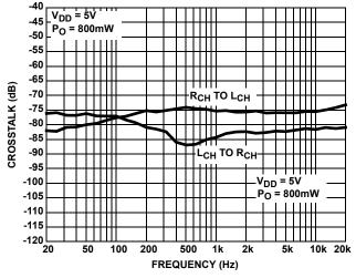
FIGURE 5. CROSSTALK vs FREQUENCY
