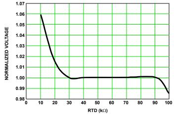
FIGURE 5. TIMING CAPACITOR VOLTAGE vs RTD
