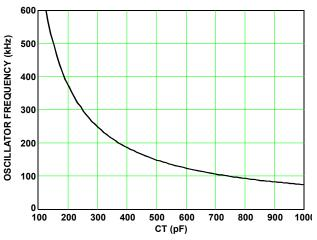
FIGURE 3. CAPACITANCE vs OSCILLATOR FREQUENCY (RTD =  $49.9k\Omega$ )
