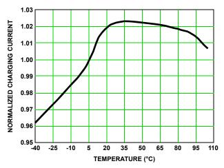
FIGURE 4. CHARGE CURRENT vs TEMPERATURE
