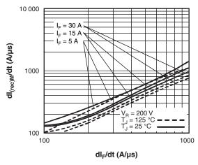
Fig. 8 - Typical  $dI_{(rec)M}/dt$  vs.  $dI_F/dt$
