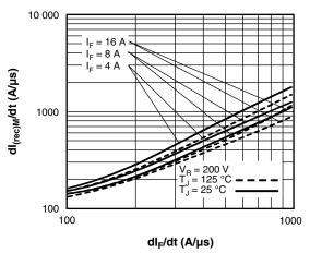
Fig. 8 - Typical  $dl_{(rec)M}/dt$  vs.  $dl_F/dt$
