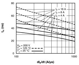
Fig. 5 - Typical Reverse Recovery Time vs. dI<sub>F</sub>/dt
