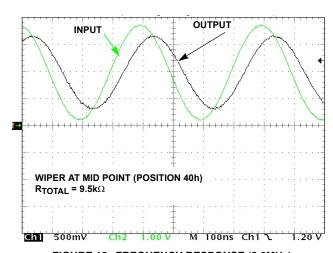
FIGURE 12. FREQUENCY RESPONSE (2.6MHz)
