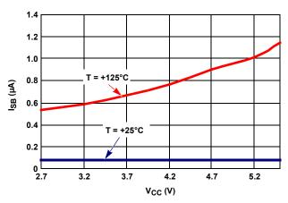
FIGURE 2. STANDBY  $I_{CC}$  vs  $V_{CC}$
