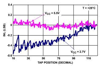
FIGURE 8. INL vs TAP POSITION IN RHEOSTAT MODE FOR  $10 \mathrm{k}\Omega$  (W)
