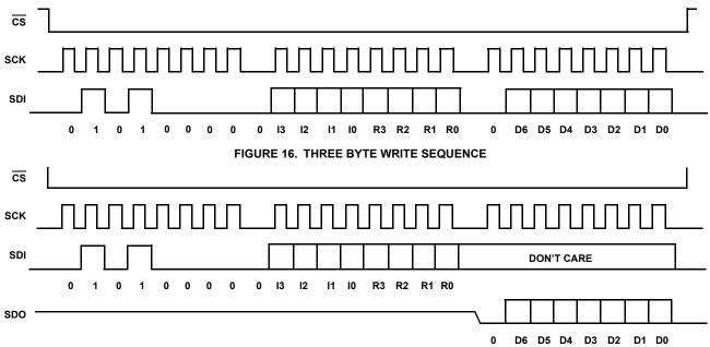
FIGURE 17. THREE BYTE READ SEQUENCE
