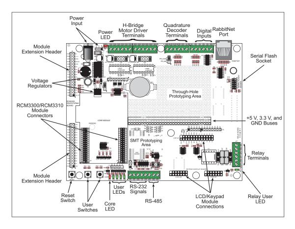
Figure B-1. Prototyping Board
