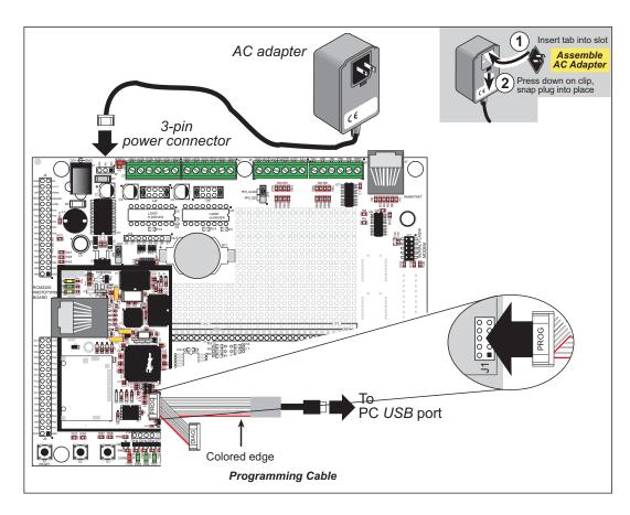
Figure 3(a). Connect Programming Cable and Power Supply
