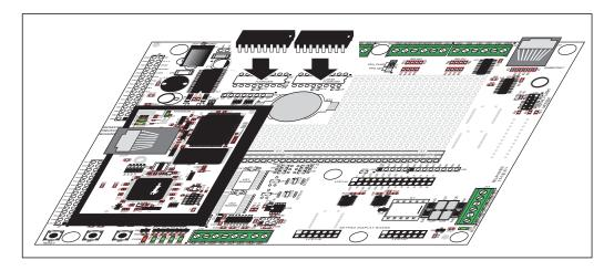
Figure B-10. Install Four-Channel Push-Pull Driver Chips
