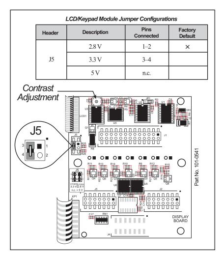
Figure C-3. LCD/Keypad Module Contrast Adjustments
