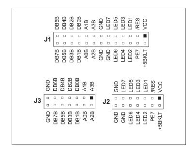
Figure C-6. LCD/Keypad Module Pinouts
