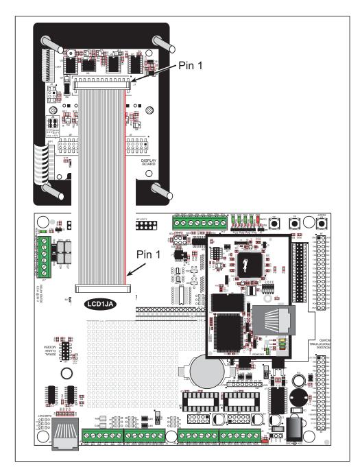
Figure C-10. Connecting LCD/Keypad Module to Prototyping Board
