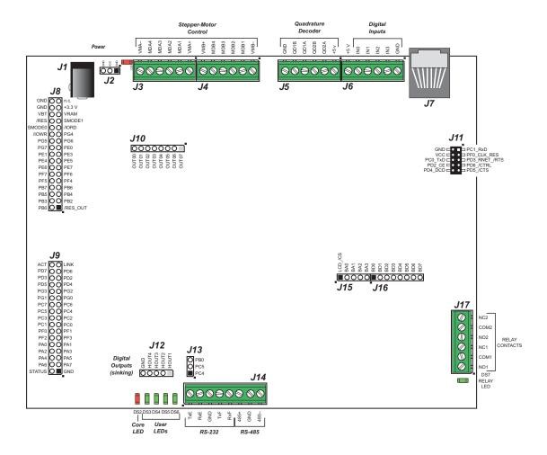
Figure B-4. Prototyping Board Pinout
