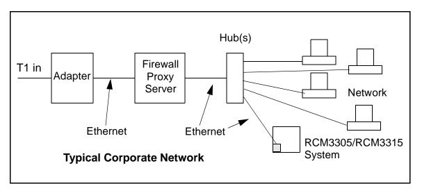
If your system administrator can give you an Ethernet cable along with its IP address, the netmask and the gateway address, then you may be able to run the sample programs without having to setup a direct connection between your computer and the RCM3305/RCM3315. You will also need the IP address of the nameserver, the name or IP address of your mail server, and your domain name for some of the sample programs.
