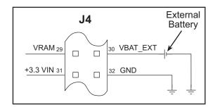
Figure D-1. External Battery Connections at Header J4
