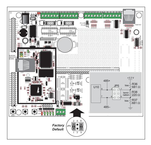
Figure B-9. RS-485 Termination and Bias Resistors
