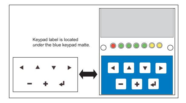
Figure C-5. Removing and Inserting Keypad Label
