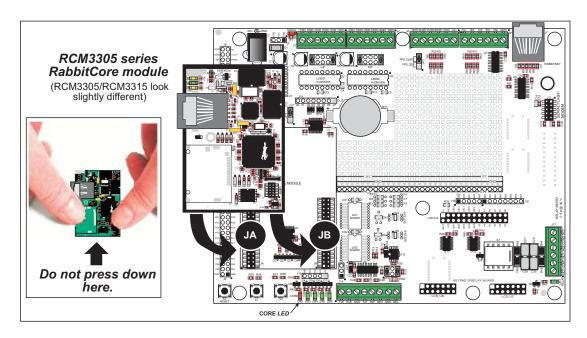
Figure 2. Install the RCM3305/ Series Module on the Prototyping Board
