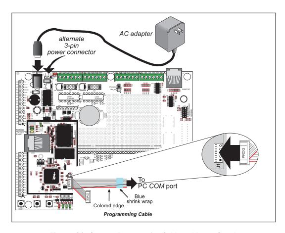
Figure 3(b). Connect Programming Cable and Power Supply
