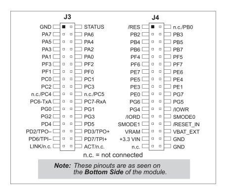
Figure 5. RCM3305/RCM3315 Pinouts
