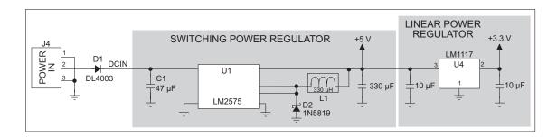
Figure B-3. Prototyping Board Power Supply
