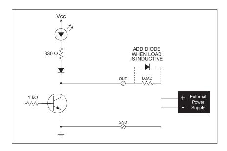
Figure B-6. Prototyping Board Sinking Digital Outputs
