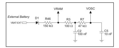
Figure D-2. RCM33305/RCM3315 Backup Battery Circuit
