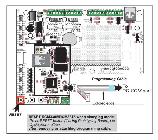
Figure 8. Switching Between Program Mode and Run Mode
