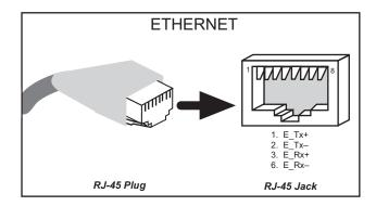
Figure 7. RJ-45 Ethernet Port Pinout
