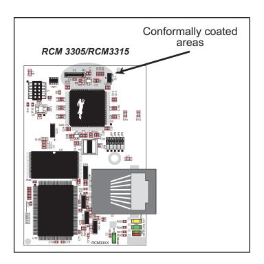
Figure A-6. RCM3305/RCM3315 Areas Receiving Conformal Coating
