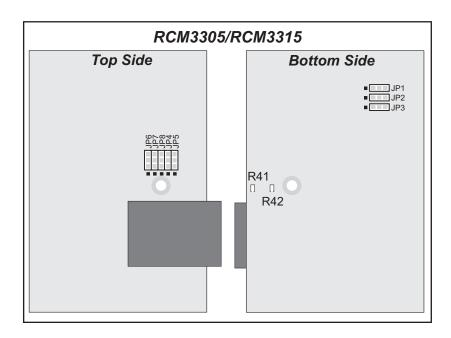
Figure A-5. Location of RCM3305/RCM3315 Configurable Positions
