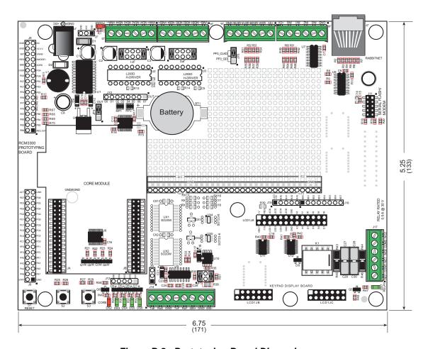
Figure B-2. Prototyping Board Dimensions
