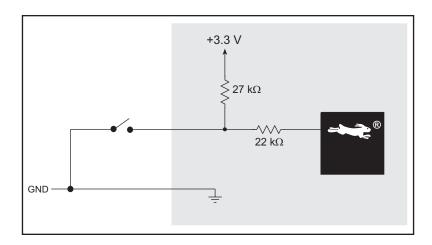
Figure B-5. Prototyping Board Digital Inputs
