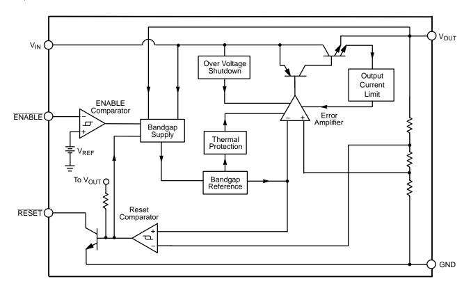
Figure 1. Block Diagram - TO-220-5
