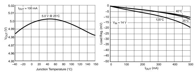
Figure 2. Output Voltage vs. Temperature
