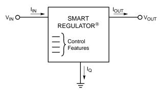
Figure 15. Single Output Regulator With Key Performance Parameters Labeled
