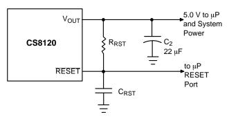
Figure 12. RC Network for RESET Delay Circuitry
