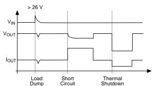
Figure 10. Typical Circuit Waveforms for Output Stage Protection
