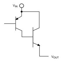
Figure 9. Composite Output Stage of the CS8120
