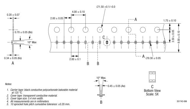
Figure 6. SMS7621-092 Tape and Reel Dimensions
