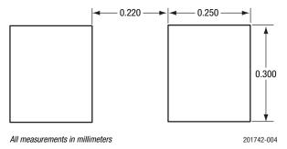
Figure 4. SMS7621-092 Suggested Stencil Aperture
