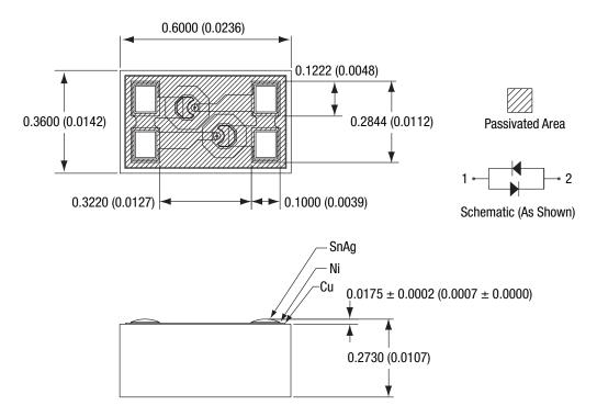
All measurements in millimeters (inches shown in parentheses). Unless otherwise specified, all dimensions are  $\pm$  0.025 mm ( $\pm$ 0.001 in.).
