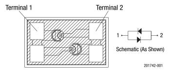
Figure 1. SMS7621-092 Pinout (Bottom View)
