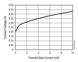
Figure 2. Forward Voltage vs Forward Current (Ts = 25  $^{\circ}$ C)
