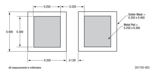
Figure 3. SMS7621-092 PCB Layout Footprint
