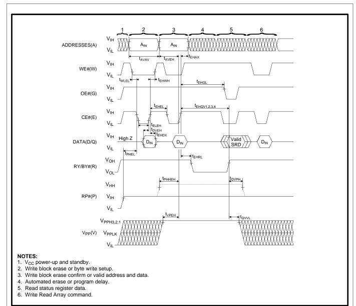
Figure 17. AC Waveform for CE#-Controlled Write Operations
