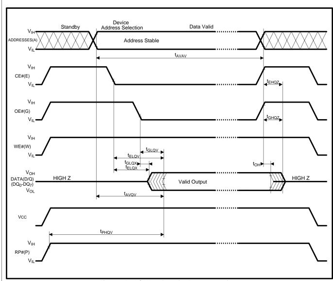
Figure 15. AC Waveform for Read Operations
