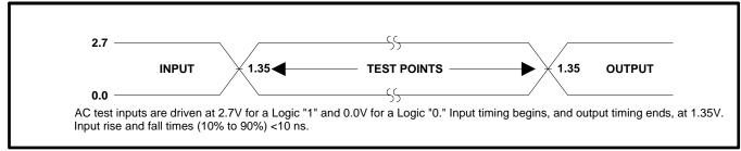
Figure 11. Transient Input/Output Reference Waveform for V<sub>CC</sub>=2.7V-3.6V
