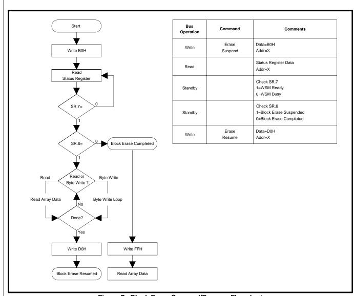
Figure 7. Block Erase Suspend/Resume Flowchart
