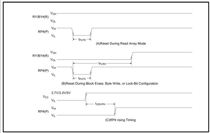
Figure 18. AC Waveform for Reset Operation
