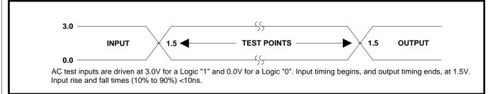
Figure 12. Transient Input/Output Reference Waveform for V<sub>CC</sub>=3.3V±0.3V and V<sub>CC</sub>=5V±0.25V (High Speed Testing Configuration)
