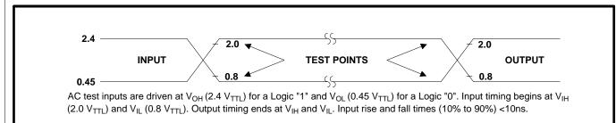
Figure 13. Transient Input/Output Reference Waveform for V<sub>CC</sub>=5V±0.5V (Standard Testing Configuration)
