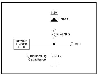
Figure 14. Transient Equivalent Testing Load Circuit
