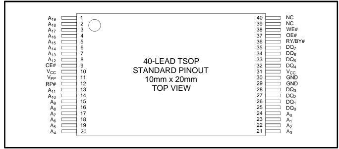
Figure 2. TSOP 40-Lead Pinout
