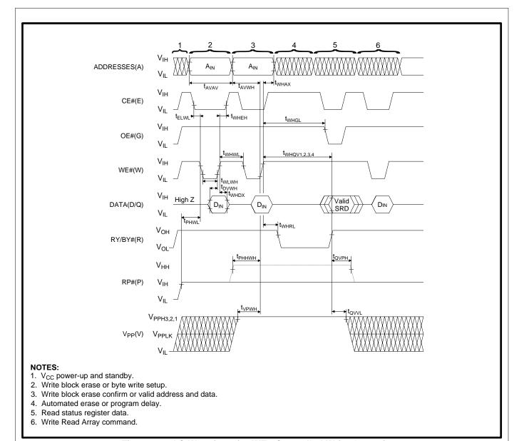
Figure 16. AC Waveform for WE#-Controlled Write Operations
