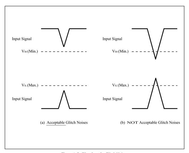
Figure A-2. Waveform for Glitch Noises
