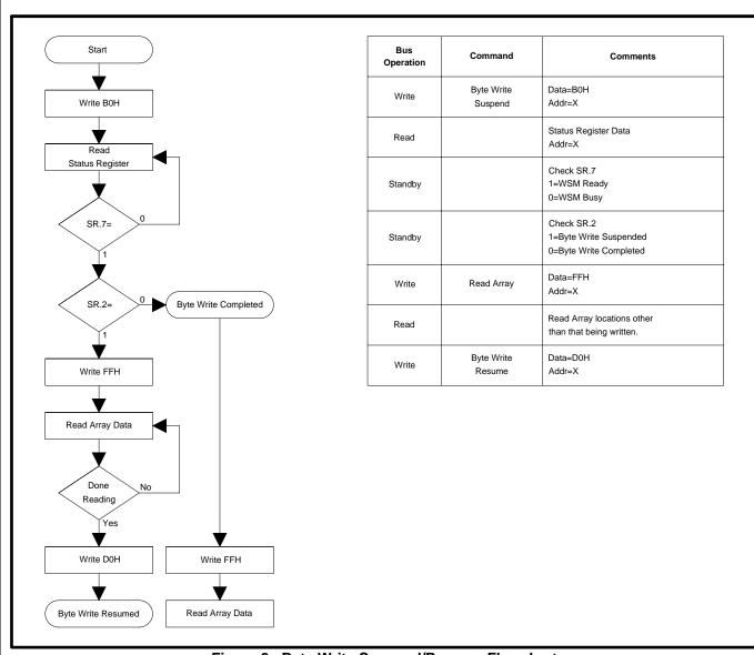
Figure 8. Byte Write Suspend/Resume Flowchart
