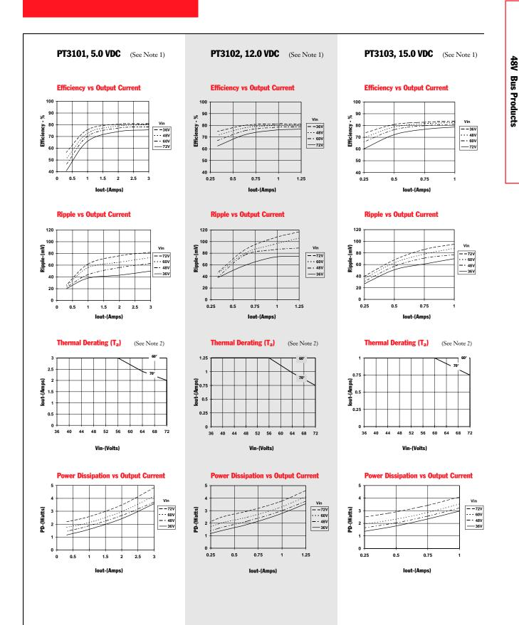
Note 1: All data listed in the above graphs, except for derating data, has been developed from actual products tested at 25°C. This data is considered typical data for the DC-DC Converter. Note 2: Thermal derating graphs are developed in free air convection cooling of 40-60 LFM.
