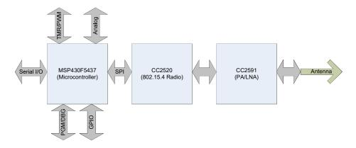
Figure 1 ProFLEX01 Module Block Diagram - High-Level
