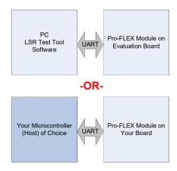
Figure 8 Host Microcontroller Modes of Operation
