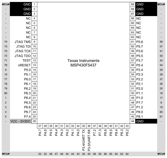
**Figure 3 Module Pinout**
