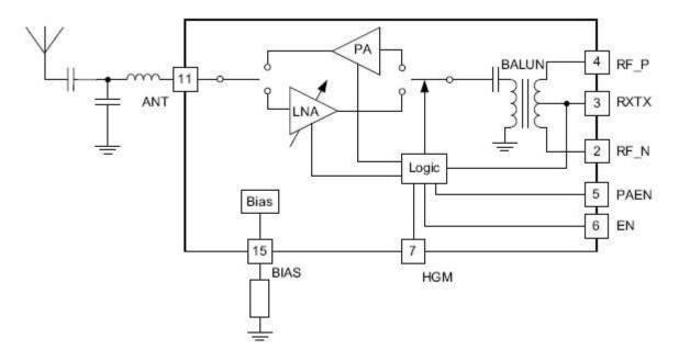
Figure 7 CC2591 Block Diagram
