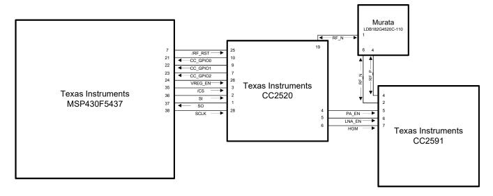
Figure 4 ProFLEX01 Module Block Diagram - Internal Interconnects
