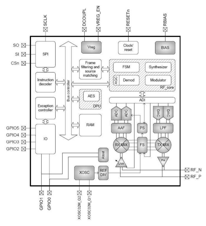
Figure 6 CC2520 Block Diagram
