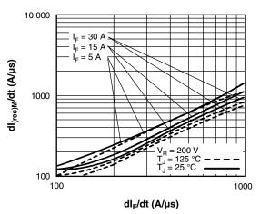
Fig. 8 - Typical  $dI_{(rec)M}/dt$  vs.  $dI_F/dt$
