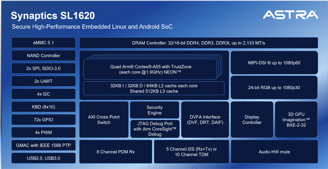
Figure 1. Astra SL1620 high-level block diagram
