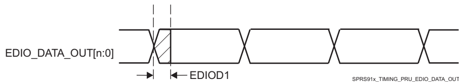
Figure 5-63. PRU-ICSS EDIO DATA_OUT Timing
