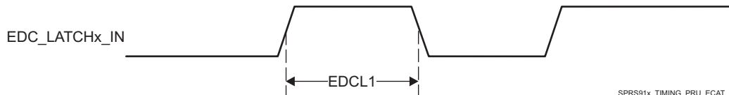
Figure 5-62. PRU-ICSS ECAT LATCHx_IN Timing
