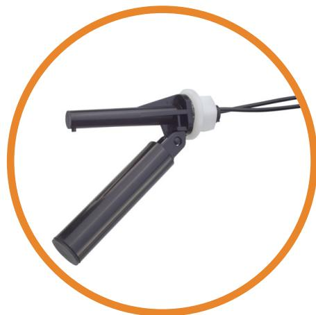
The RSF30 is a higher power side entry, internally fitted switch. These may be used for directly switching some small loads of less than 100VA. Fitting of this type requires access to the inside of the tank.
