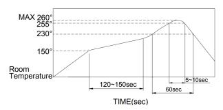
■ The condition noted above is the temperature of the copper foil on the surface of the PCB. There are cases where the temperature of the board greatly differs from the surface of the switch. Do not allow the surface temperature of the switch to exceed 260°C.
