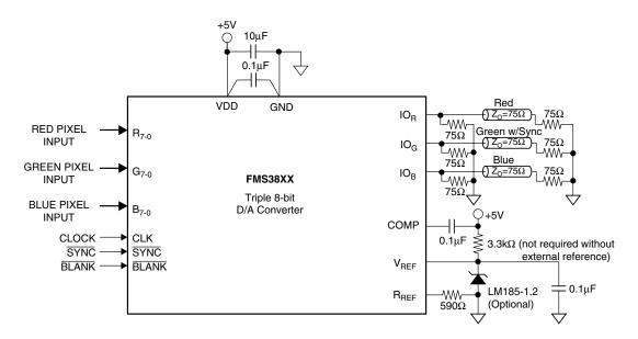
Figure 4. Typical Interface Circuit
