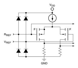
Figure 3. Equivalent Analog Input Circuit
