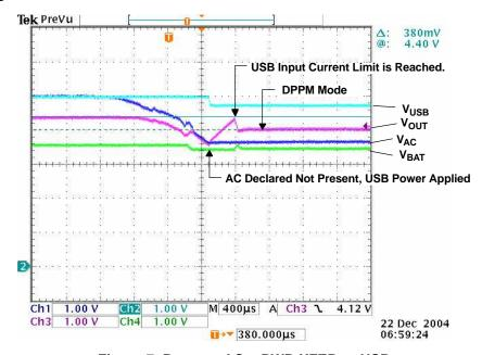
Figure 7. Remove AC – PWR XFER to USB
