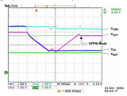
Figure 8. Remove AC (Low Battery) – PWR XFER to USB
