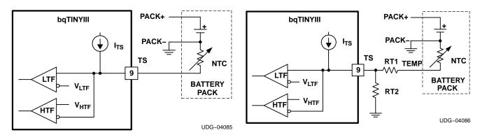
Figure 14. TS Pin Configuration
