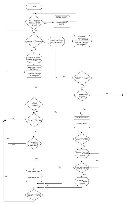
Figure 3. Charge Control Operational Flow Chart
