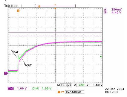
Figure 12. Insert Battery – Power-Up Output via BAT
