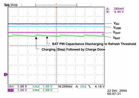
Figure 11. Battery Absent - PWR XFER to USB
