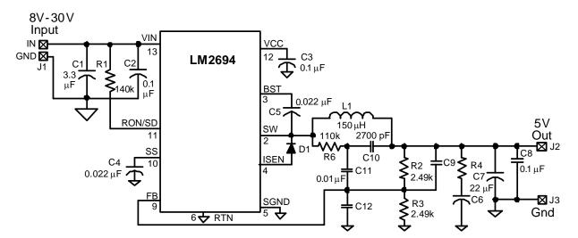
Figure 5. Evaluation Board Schematic
