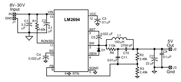
Figure 2. Minimum Output Ripple Configuration
