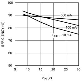
Figure 7. Efficiency vs Input Voltage
