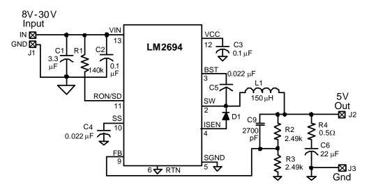
Figure 3. Intermediate Ripple Configuration
