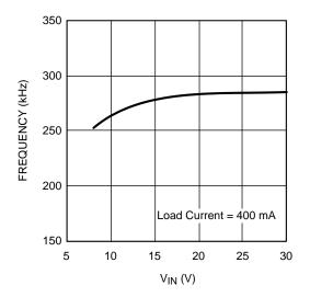
Figure 9. Switching Frequency vs. Input Voltage
