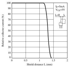
Fig.12 Relative Collector Current vs. Shield Distance (2)
