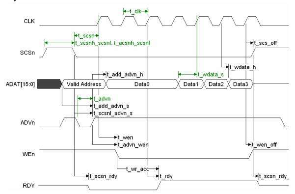
Note: RDY going low is asynchronous to t\_scsn\_rdy. Going high, it is synchronous to CLK. Valid Data Time programmable through Device Wait Count Register. For Wait Count values other than 0 or 1 (when DMAREQ is used), t\_wr\_acc = Wait Count + 1.
