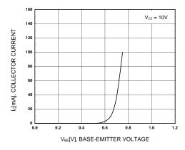
Figure 5. Base-Emitter On Voltage
