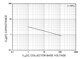
Figure 7. Reverse Transfer Capacitance
