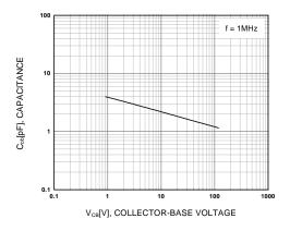
Figure 6. Collector Output Capacitance
