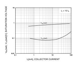
Figure 4. Base-Emitter Saturation Voltage Collector-Emitter Saturation Voltage
