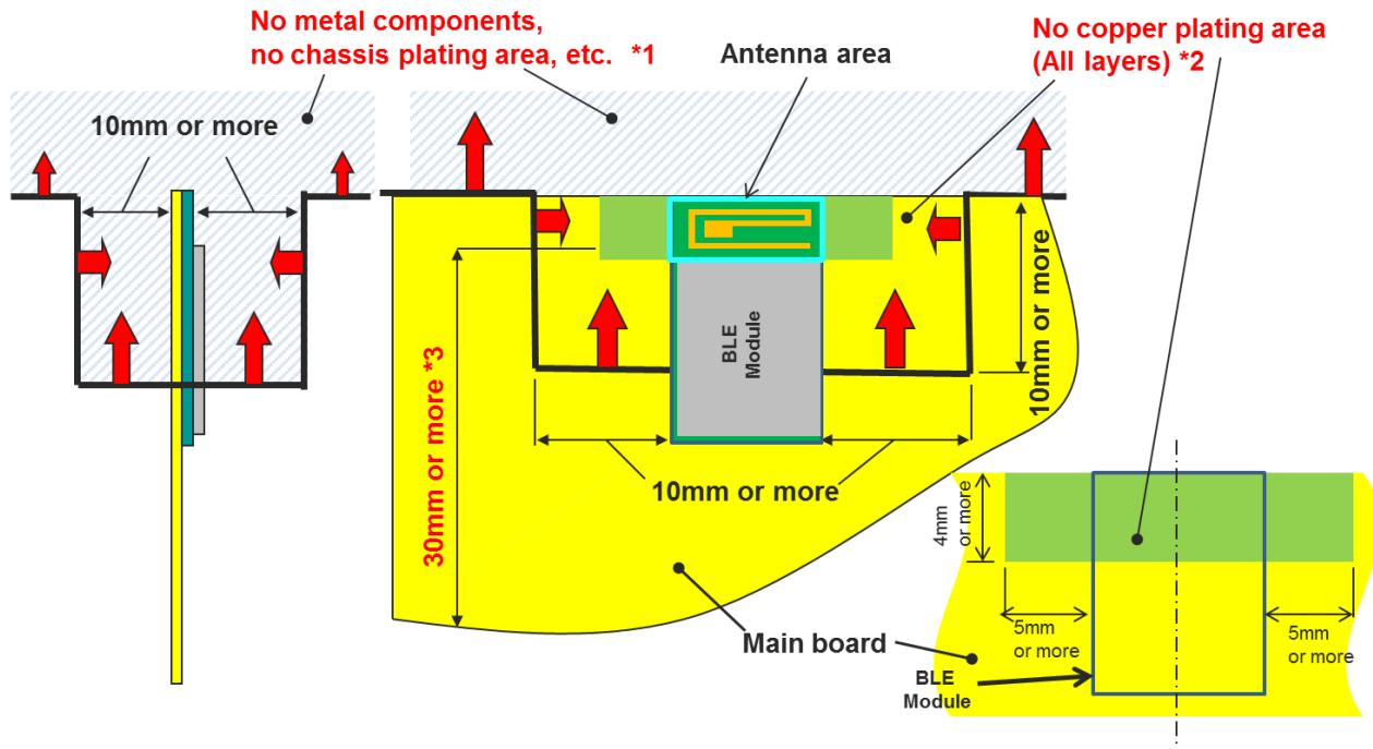
1 Please do not place any metal components in **blue shaded space.\*1**) We do not recommend placing any metal objects upper space of the module in the above figure. If it needs to place metal objects, please consider keeping the metal off from the antenna as far as you can. Such as signal line and metal chassis as possible except for main board while mounting the components in \*1 space on the main board is allowed except for no copper plating area. (\*2).
