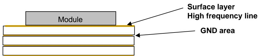
GND pattern of each layer should be connected to GND area with large number of via.
