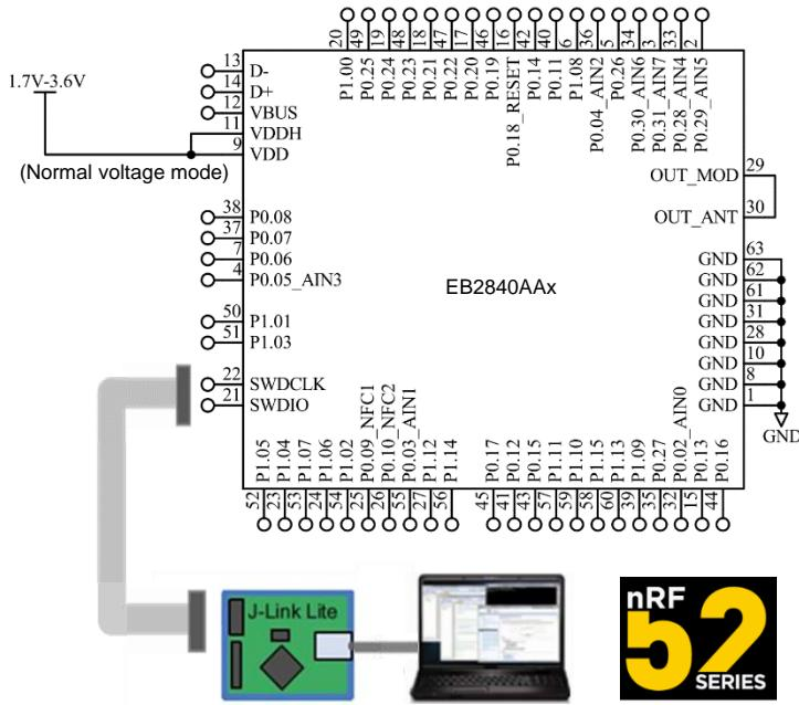
SWD (Serial Wire Debug) is a high performance 2-pin debug port that replaces JTAG. You can debug and program with J-link Lite. When using J-LINK Lite, it is convenient to mount a socket on the customer's main board. The socket will be "10-pin connector two rows of 1.27mm pitch (Ex: PSS-720153-05, Hirosgui instrument). J-Link Lite operates at 3.3 V. do not operate at 1.8 V, so please be careful.
