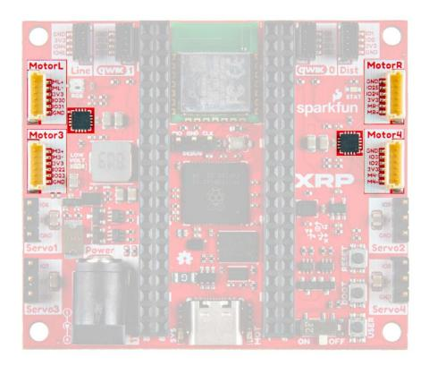
The term H-bridge comes from how this circuit design looks on a schematic diagram. It has four internal switches that control whether the motor spins Clockwise (CW), Counter Clockwise (CCW), Coasts (no drive power), and Stops. When going through the XRP Kit curriculum you'll learn how to program the robot to tell the motor drivers to control the motors' speed and direction.
