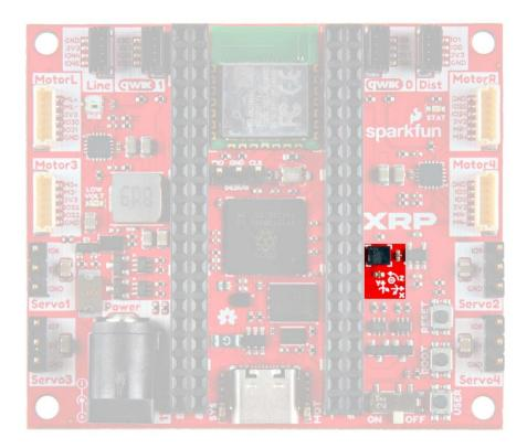
The accelerometer in this chip has four measurement ranges of  $\pm 2/\pm 4/\pm 8/\pm 16$  g. These ranges allow you to customize the limits of the acceleration forces measured. The gyroscope has five selectable measurement ranges of  $\pm 125/\pm 250/\pm 500/\pm 1000/\pm 2000$  DPS (degrees per second). Refer to the silk screen symbols on the XRP Controller for the directions of each axis.
