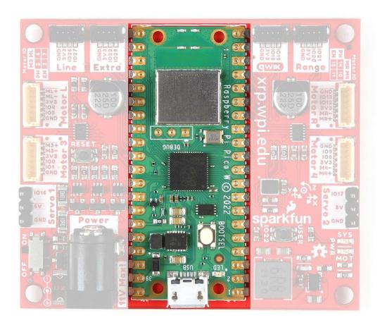
Think of the Pico W as a brain sending signals to other parts of the "body" to tell them what to do. It has several General Purpose Input/Output (GPIO) pins that connect to the other major parts on this board so it can send and receive data from them and return it to you visually (such as seeing the motors move) or virtually (such as watching data on a computer monitor).
