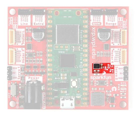
The accelerometer in this chip has four measurement ranges of  $\pm 2/\pm 4/\pm 8/\pm 16$  g. These ranges allow you to customize the limits of the acceleration forces measured. The gyroscope has five selectable measurement ranges of  $\pm 125/\pm 250/\pm 500/\pm 1000/\pm 2000$  DPS (degrees per second).
