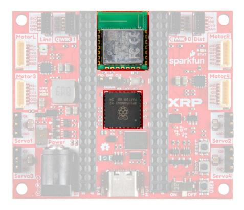
Think of the RP2350 as a brain sending signals to other parts of the "body" to tell them what to do. It has several General Purpose Input/Output (GPIO) pins that connect to the other major parts on this board so it can send and receive data from them and return it to you visually (such as seeing the motors move) or virtually (such as watching data on a computer monitor).
