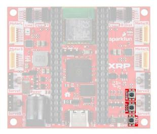
The USER button connects to GPIO36 on the RP2350 which allows it to be programmed for various purposes. The RESET button does just what its name suggests and resets the entire board when pressed. This can help to reboot the robot or to restart a sequence you want the Robotics Kit to perform. Holding the BOOT button either when plugging in a USB cable or when pressing the RESET button sets the RP2350 to behave as a mass storage device when connected to a computer for uploading firmware.
