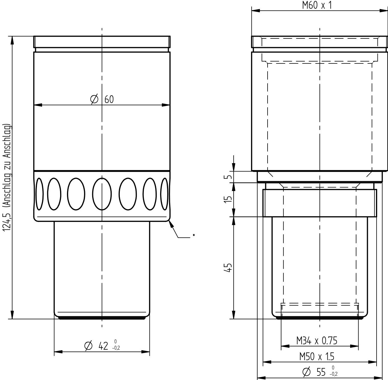
\*: clamping ring (for mounting plate with dia. 55 through hole, thickness max. 10)
